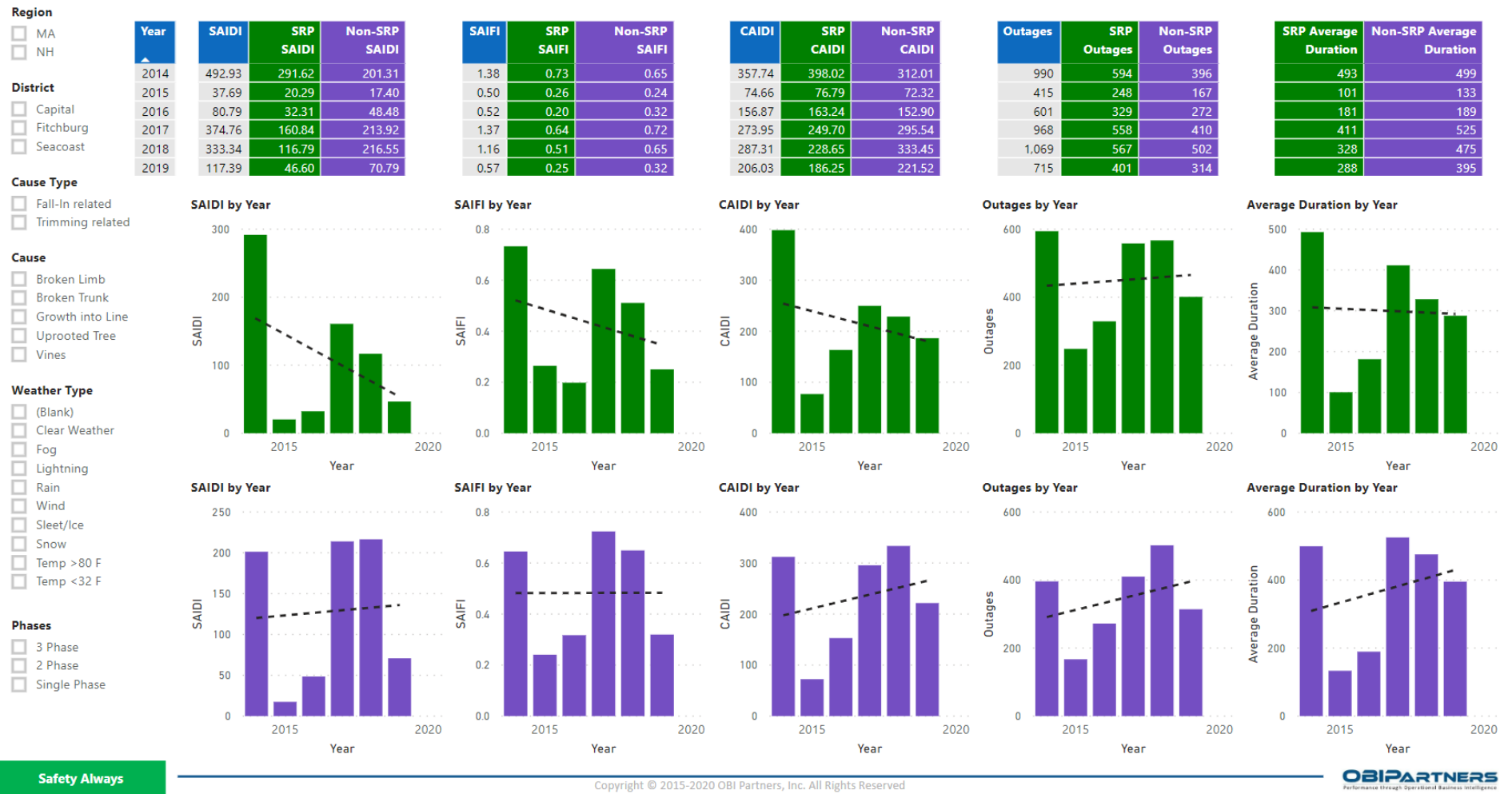
Figure 11 - SRP vs. Non-SRP Circuit Performance for All Phases and All Weather Events
