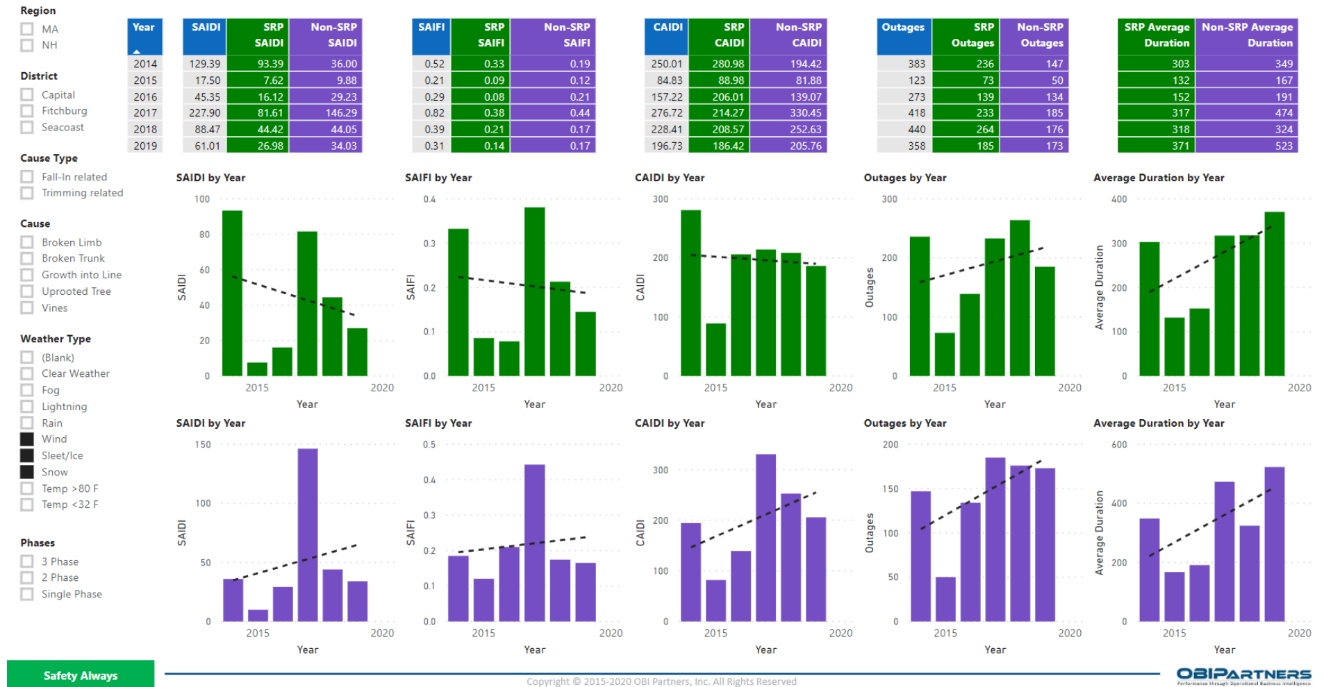
Figure 13 - SRP vs. Non-SRP Circuit Performance for All Phases and Storm Only Events
