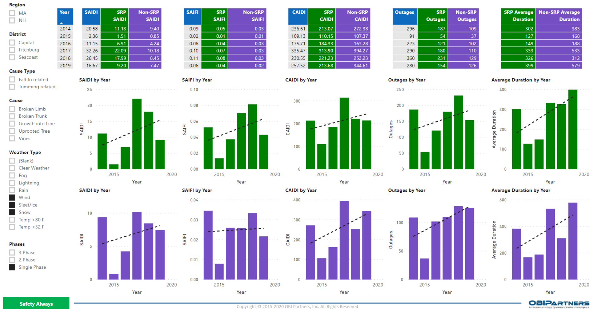
Figure 15 - SRP vs. Non-SRP Circuit Performance for Single-Phase Only and Storm Only Events
